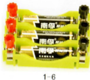
Fig. 1-6: Battery boxes are connected in parallel to form a battery pack with a more capacity and intensity of a current
