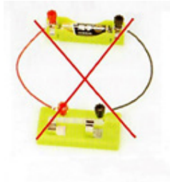
Fig. 1-3 Shortcircuit, damage of a battery
